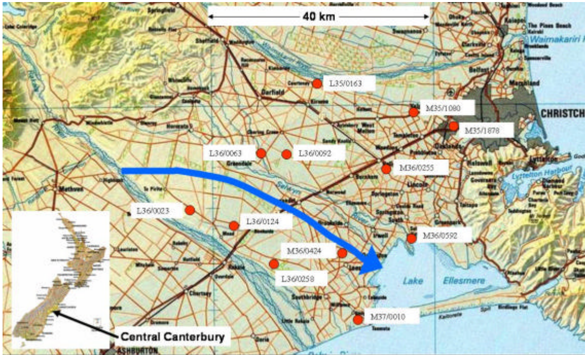
Figure 1. Central Canterbury, showing the locations of long-term observation wells and an example groundwater flow path (curved arrow) from the Rakaia River to Lake Ellesmere.
